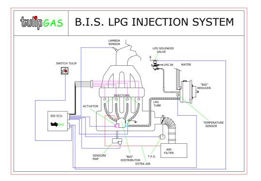
LPG fuel consumption by the "BIS" system is lower than the other, more conventional systems, because of a better control of the precise quantity of gas needed under all conditions of the engine.
