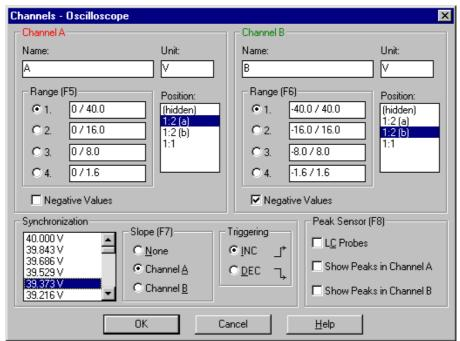
The **"Synchronization"** settings let you choose the channel, with which the displaying of the graphs should be synchronized, and the level, crossing of which should make drawing
