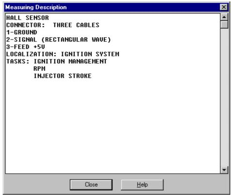
If the configuration containing a description is loaded, the window with the description will be displayed. If you close it, you can make the measurements.
