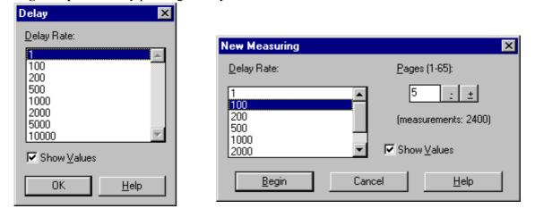
The program counts the delay for "**recorder**" and "**diagnoskop**" modes in a form of measurements that are skipped.
