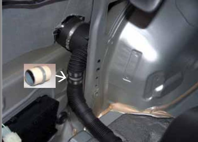
↓ ↵ [gas pipe fitting]      ↑ [lock washer]
