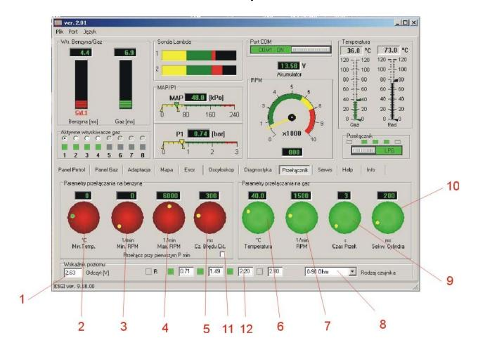
1. Voltage readout from the LPG level gauge in the tank
