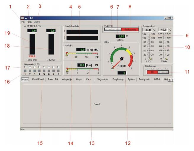
The main window is always visible irrespective of chosen setting or readouts and allows to control constantly all the necessary engine parameters during the change of setting or adaptation.
