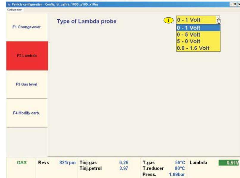
For the self-calibrating system to operate it is not necessary that the lambda sensor be connected. Connection is required only in order to display its operation and has no influence whatsoever on carburetion. If the 4-wire lambda sensor is connected, this menu permits setting the type. Select among: ① 0-1 Volt; 0-5 Volt; 5-0 Volt, 0.8-1.6 Volt.
