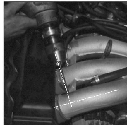
Pic. 31 - Manifold drilling
