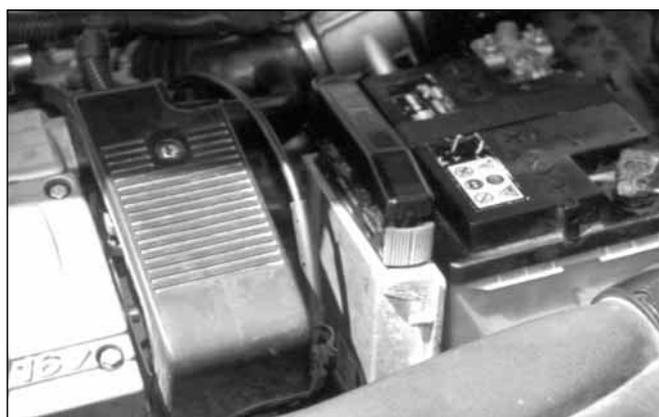
Pic. 37 ECU assembling in the engine compartment
