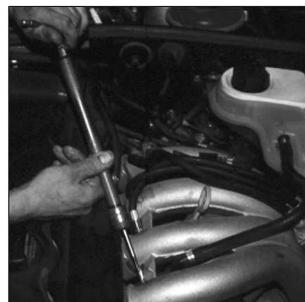
Pic. 32 - Manifold threading
