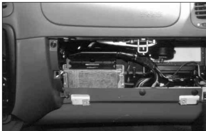
Pic. 36 ECU assembling in the passenger compartment
