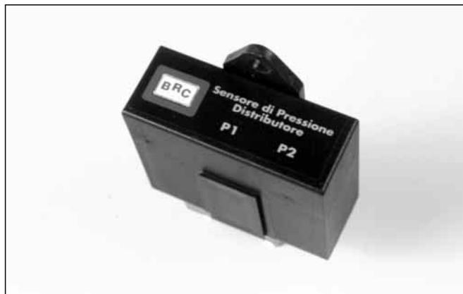
Pic. 19 Smart distributor pressure sensor
